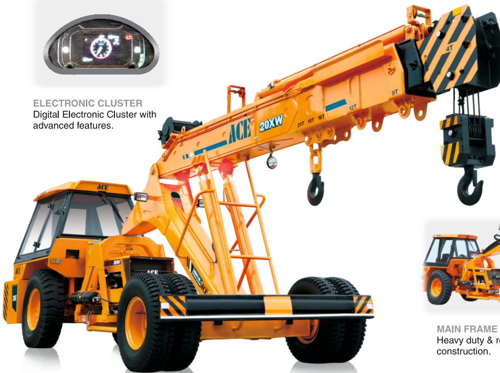
ACE 20XW 5-Part Boom (24.6 mtrs. height) Max. Capacity Manual Extension : 2 Tonnes
