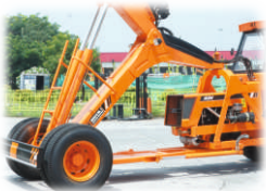
STEERING CYLINDERS 700 mm stroke cylinders ensure proper steering even in loose, sandy & rocky terrains.
