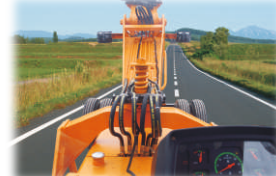
INCREASED VISIBILITY Bigger size front windscreen and re-routing of hoses provide much better front visibility.
