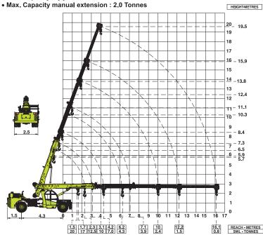
NOTE: • Rated loads are on the basis of operation on firm and level surface. Full rated lifting capacity available in articulated / steered condition.
