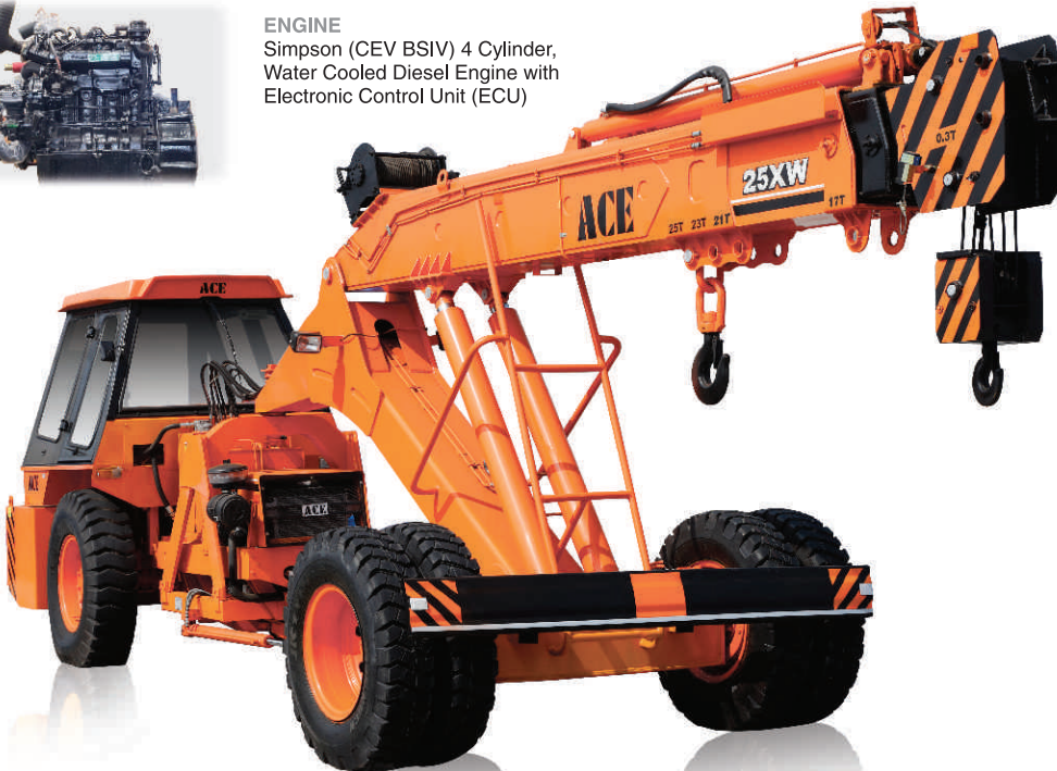
ACE 25XW 5-Part Boom (23.1 Mtrs. Height) Max. Capacity Manual Extension : 2 Tonnes
