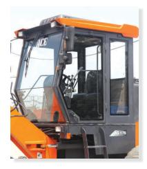
Ergonomically designed diamond shaped Air -Conditioned cabin with wide-view vision, FM Radio, adjustable operator seat & operating console. The rollover protective structure (ROPS) is designed as per ISO 3471-1994, ISO 3164-1995 (E) standards providing water, dust and noise resistance for operator's comfort and safety.
