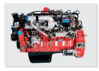
Ashok Leyland H-series 6 cylinder water cooled Turbocharged Diesel engine with SCR technology generating 180 hp @ 2200 rpm meeting CEV Stage-V emission compliance. Common Rail Fuel System for effective power strokes and efficient fuel consumption. This high torque engine provides high pushing power and thus improves operating efficiency.
