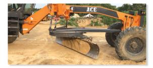
$360^{\circ}$  rotation of the blade also ensures productivity during reverse movement of the grader, specially in heap breaking application. Offers high productivity in minimum no. of passes saving fuel, time and maintenance cost.
