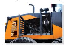
Open vents from either side ensures easy access for daily maintenance checks, serviceability and adequate ventilation.
