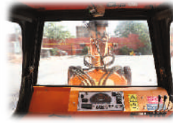
INCREASED VISIBILITY Bigger size front windscreen and re-routing of hoses provide much better front visibility.
