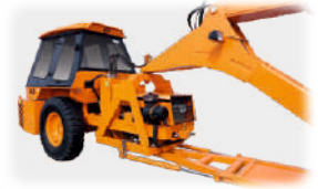
STEERING CYLINDERS 880 mm stroke cylinders ensure proper steering even in loose, sandy & rocky terrains.
