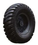
Heavy duty Rock grade tyres of size 14.00 X 25 with 20 Ply rating for minimum wear and increased life. 14.00 x 24 with 16 PR for road applications.
