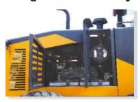
Open vents from either side ensures easy access for daily maintenance checks, serviceability and adequate ventilation.
