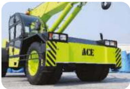
GROUND CLEARANCE Ground clearance of 350mm for easier rough terrain operation.
