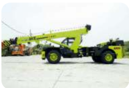
OPTIMIZED KINEMATICS AND LOW C.G. F270 crane has been designed for operational safety with low Center of Gravity (C.G.) providing best in class stability
